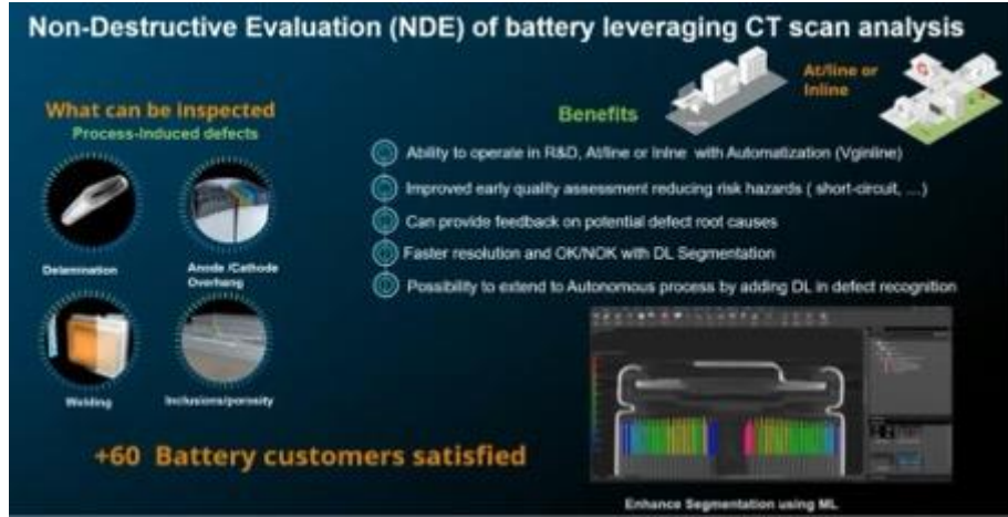
Figure 5—CT Scan Analysis Enables NDE (Courtesy of Hexagon)
