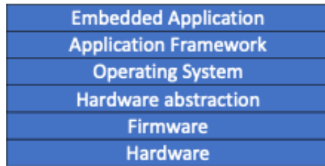
Figure 1—A Typical Hardware/Software Technology Stack (Courtesy of HCL)
