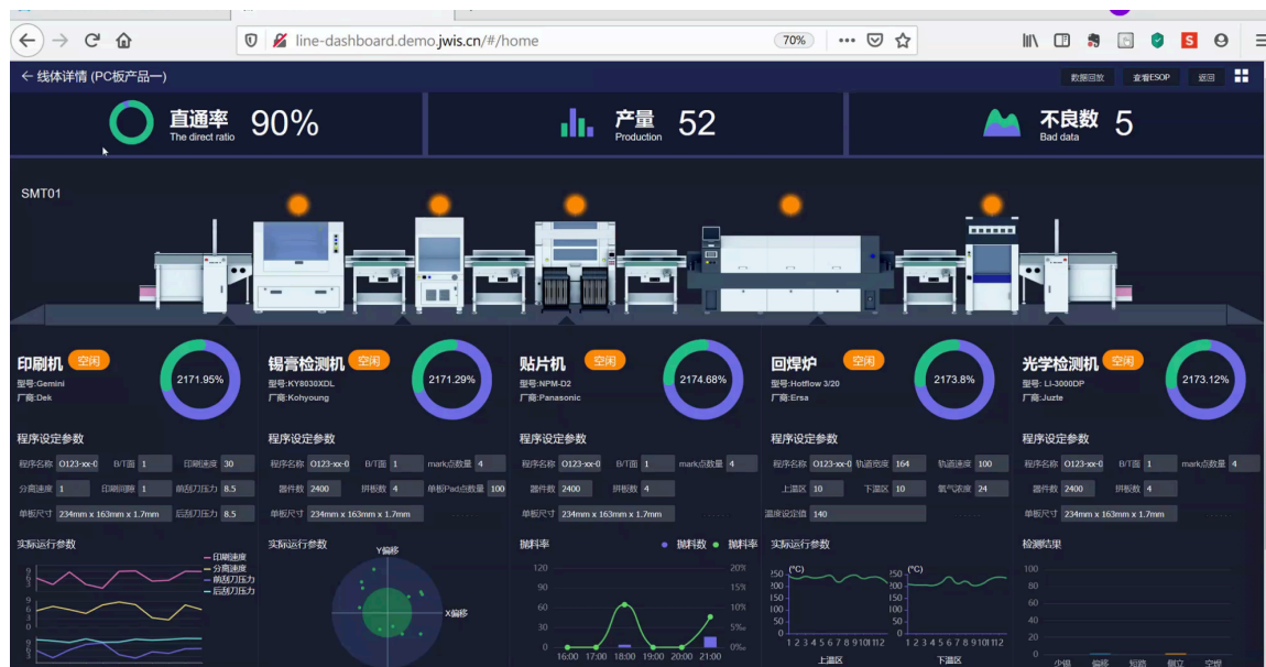
Figure 4— Production Line Digital Twin (Courtesy of JWI)
