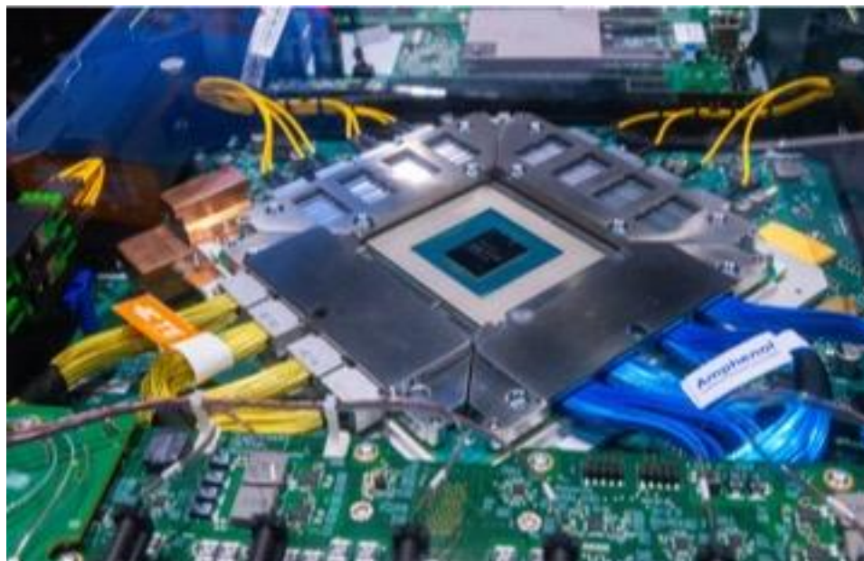
Figure 5—Wistron 32X 800GbE OSFP and 64X 400GbE optical SN switch Broadcom Tomahawk, (Courtesy of Serve the Home (STH): servethehome.com)
