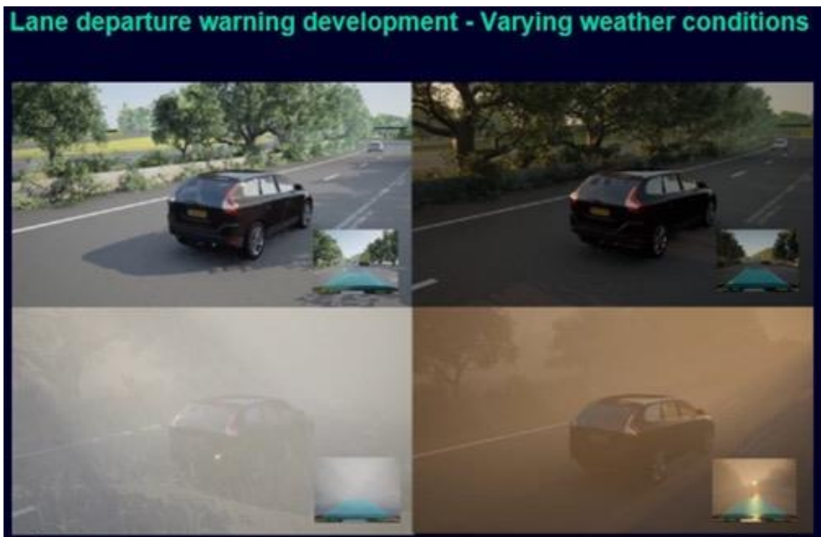
Figure 1—Scenarios Expand With Weather Variations (Courtesy of Siemens)
